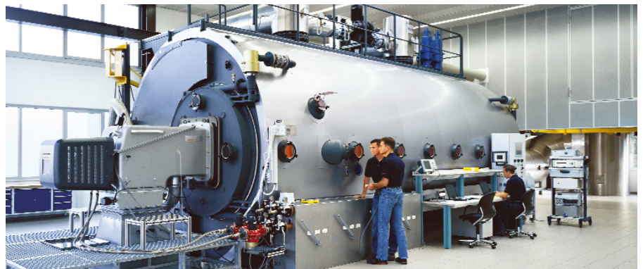
Burner with firing rate above 100,000 MBH can be tested and fired at Weishaupt testing facility
