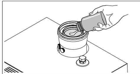
If an external siphon ① is present external to the boiler (e. g. due to the condensate hose):
