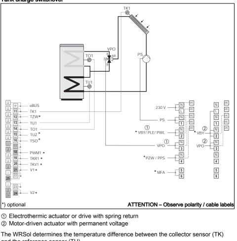
As soon as the temperature difference is greater than the set value (Switch-on difference TK - TU), the solar pump is activated, thereby charging the consumer, until the (Switch-off difference TK - TU) or the maximum temperature of the consumer has been reached. For the speed control of the solar pump PS, see chap. 8.4.
