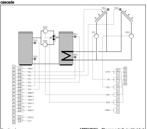
Storage tank and auxiliary tank with preliminary charge and recharge and collector
