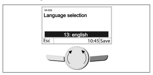
The values can be changed using a rotary knob, and the change confirmed with the **Save** key, and the next value appears.
