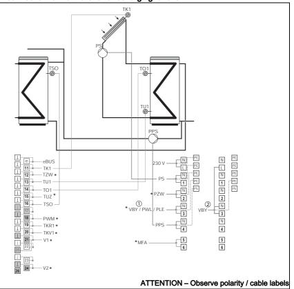
The WRSol determines the temperature difference between the collector sensor (TK) and the reference sensor (TU).
