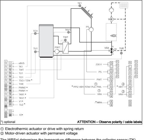
The WRSol determines the temperature difference between the collector sensor (TK) and the reference sensor (TU).
