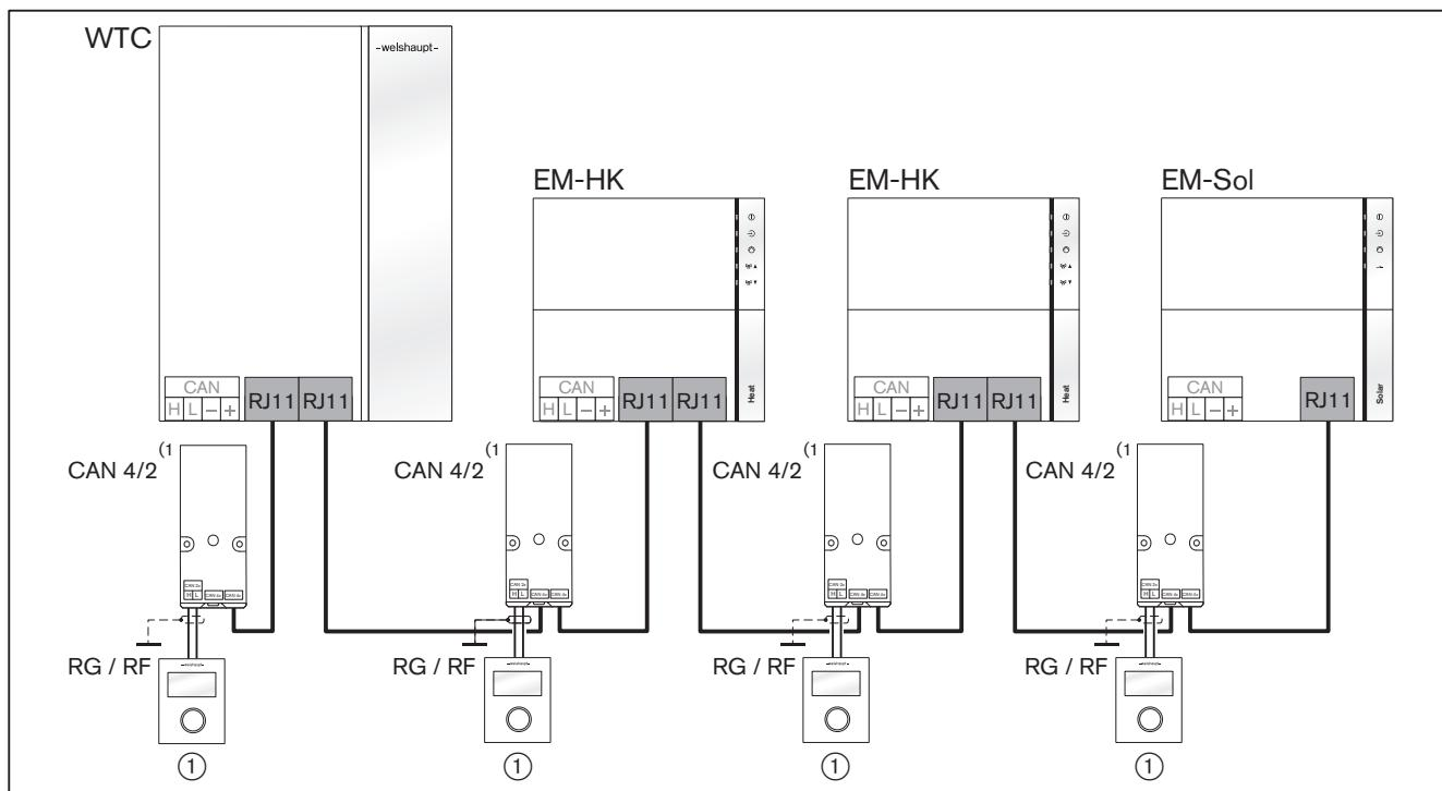
(1) max 1 room device and 2 room sensors – or – max 3 room sensors
