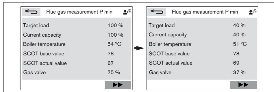
When the current capacity has reached min. load:
