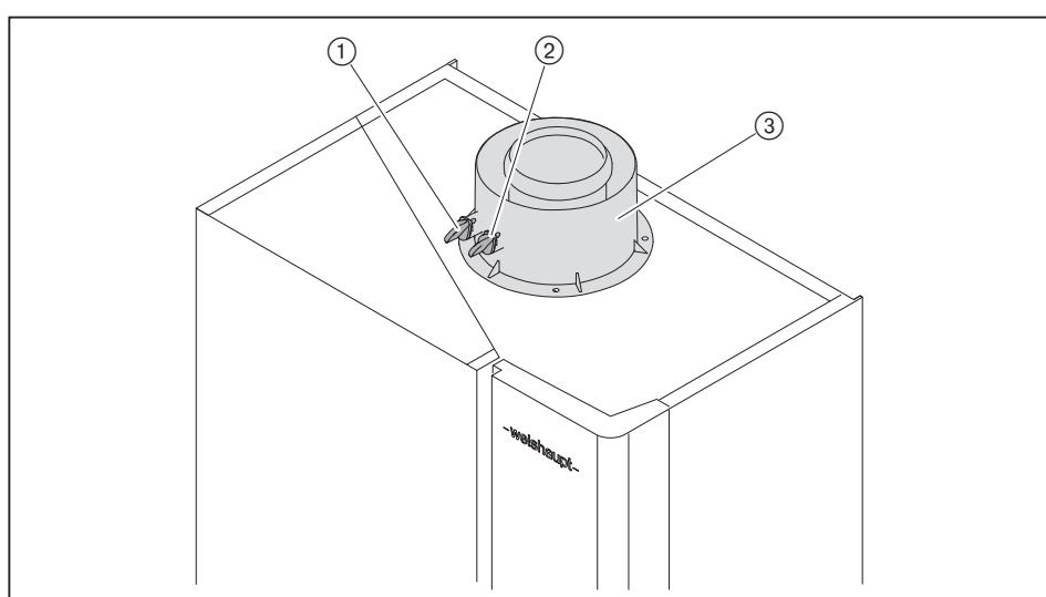
① Measuring point in supply air annular gap
