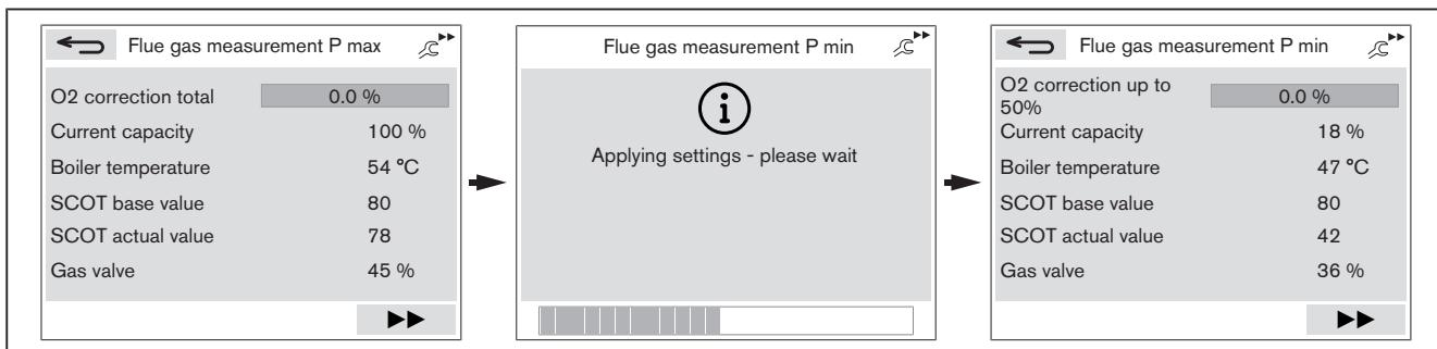
**24. Optimise O<sub>2</sub> content at min. load**
